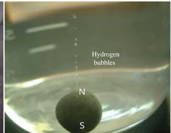
Fig. 3 The ceramic ball immersed in water showing the production of hydrogen bubbles.
